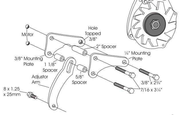
This bracket is designed to be used with the small CS 130 G.M. Alternators with the threaded mounting ear in the 2 o' clock position.
